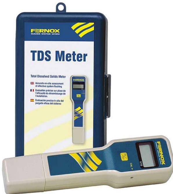
The Total Dissolved Solids ( TDS) meter offers a rapid and accurate field test for determining the concentration of total dissolved solids in system and mains waters. The prime use for the TDS meter is to determine whether a system has been correctly flushed after a chemical clean. This is done by comparing the readings between mains water and system water samples.
