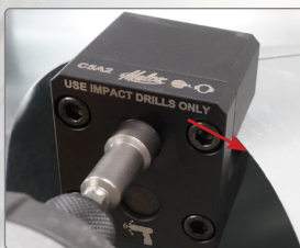
Begin crimping at angle after crease
