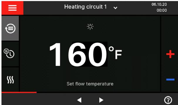
The temperature shown on the display is the boiler water temperature.
