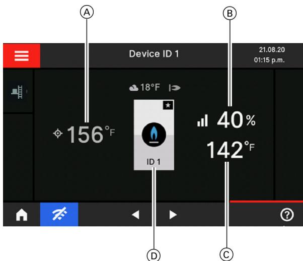
This display shows the participants in the cascade as well as the current supply temperature and the target supply temperature.
