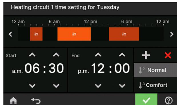
The bars in the time diagram are adjusted.
