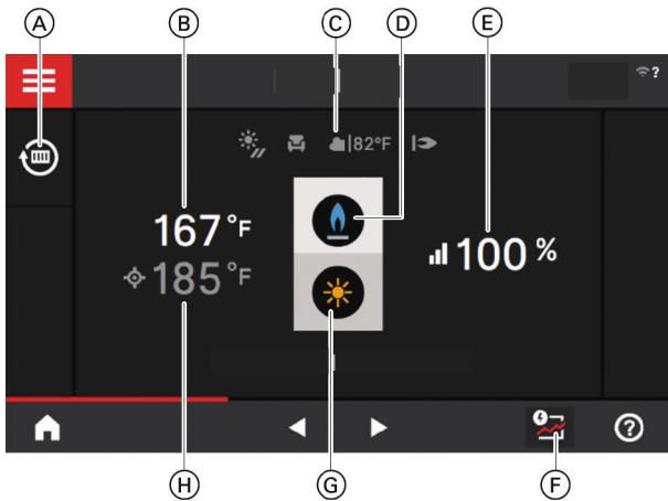
The various components present in the system are shown as graphics. Some information on the components is also provided in the default display. For more information, tap the relevant component.
