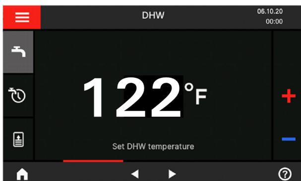
**Note:** The DHW default display is not available for systems with a storage tank with temperature switch (such as an Aquastat).
