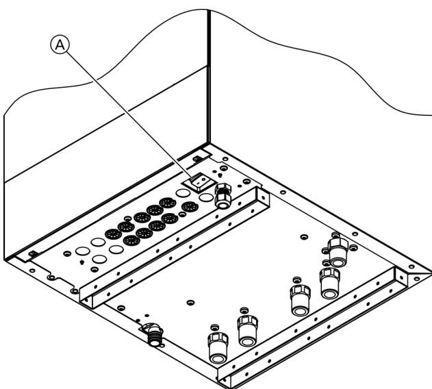
**Note:** The control unit can be located at the top or bottom.
