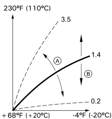
**Note:** Setting the slope or shift too high or too low will not cause any damage to your heating system. Both settings affect the level of the supply temperature, which may then be too low or unnecessarily high.
