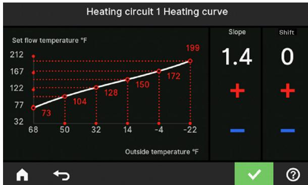
**Note:** The heating curve can only be adjusted in weather-compensated operation.
