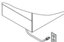
120/1/60 12A Power Supply with disconnect and protection. The Vitodens 200-W comes with a pre-installed power cord with 3 prong plug for simplified installation.
