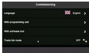
This boiler can be commissioned using the Vitoguide Mobile App or the boiler's HMI. To proceed using the app, select 'With App' to continue with the boiler's HMI setup with the programming unit.
