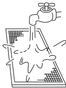
Fig. 22 —Cleaning Filter with Water or Vacuum
