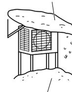
Install the unit high enough off the ground to prevent burying in snow.
