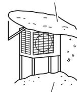
Install the unit high enough off the ground to prevent burying in snow.
