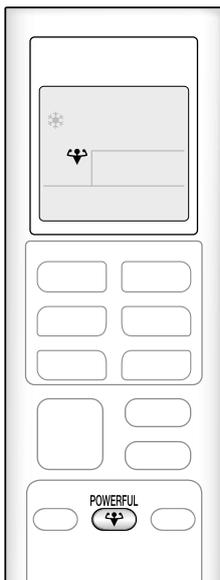
POWERFUL operation quickly maximizes the cooling (heating) effect in any operation mode. In this mode, the air conditioner operates at maximum capacity.
