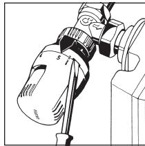
1. Turn the knob to the fully open position (Pos. 5). Using a screw-driver, unlock the ring, pressing it fully towards the valve body.
