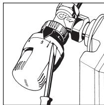
1. Using a screw-driver, unlock the ring, pressing it fully towards the valve body.
