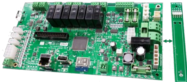
Figure 50 Separating the humidity sensor strip from the main replacement board
