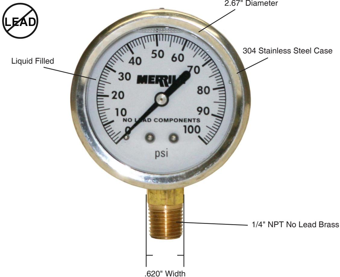
Pressure gauges are suitable for water, air, steam, and other pressure applications that will not deteriorate brass alloys. (Individually boxed.)
