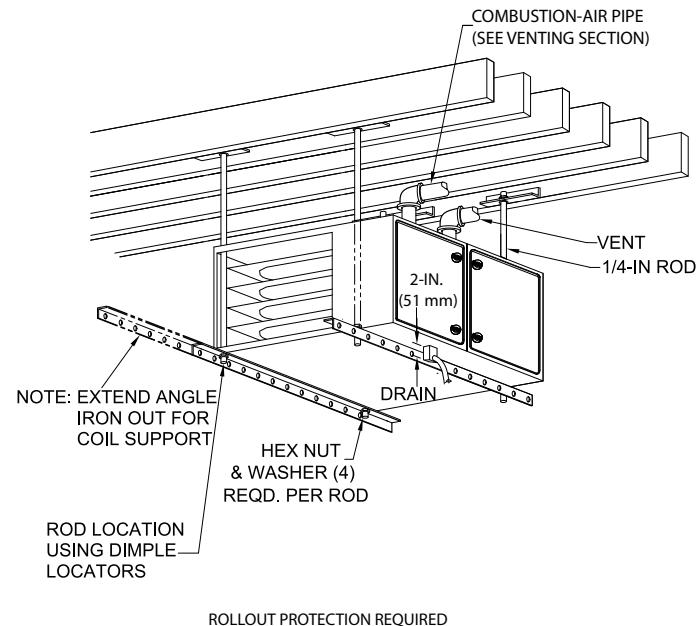
Install 12" x 22" (204 x 559 mm) sheet metal in front of and above the burner compartment area. The sheet metal MUST extend above the furnace casing by 1-in. (25 mm) with the door removed. A 1-in. (25 mm) clearance minimum between top of furnace and combustible material is required. The entire length of furnace must be supported when furnace is used in horizontal position to ensure proper drainage.
