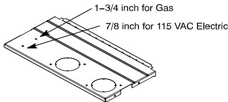
Fig. 30 – Alternate Gas and Electric Entry
