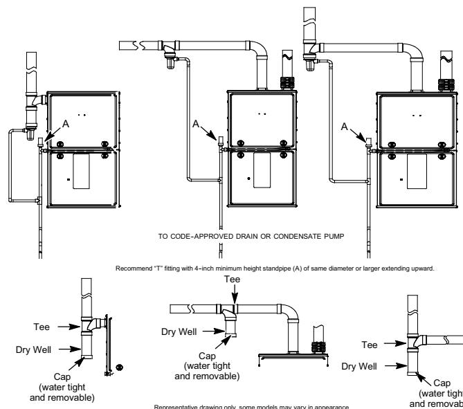
**Fig. 50 – Recommended Combustion Air Inlet Moisture Trap**
