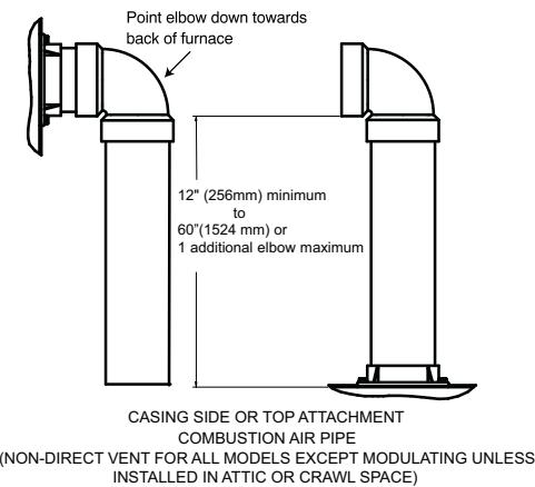
**Fig. 46 – Combustion Air Pipe Attachment**
