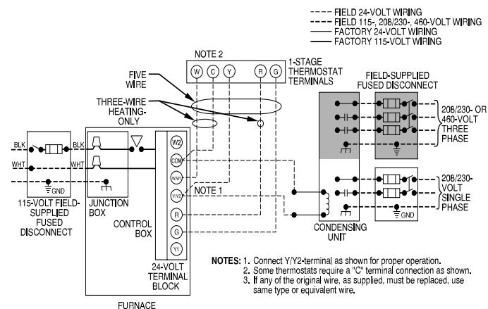
Fig. 32 – Typical Field Wiring Diagram
