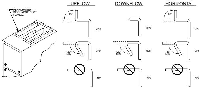
Fig. 20 – Duct Flanges
