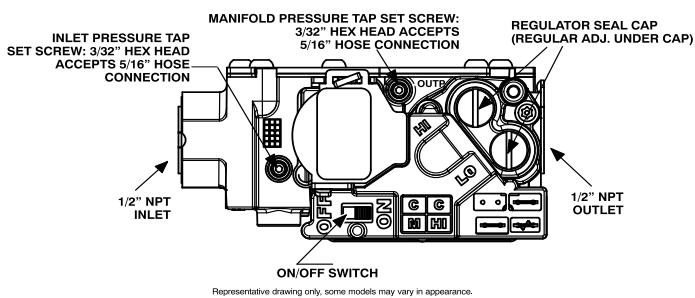
**Fig. 63 – Gas Valve with Tower Pressure Ports**
