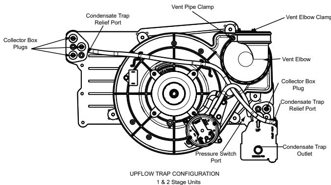
**Fig. 8 – Upflow Trap Configuration**
