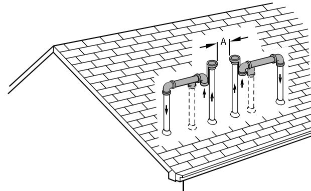
**Fig. 45 – Pipe Vent and Combustion** A96128
