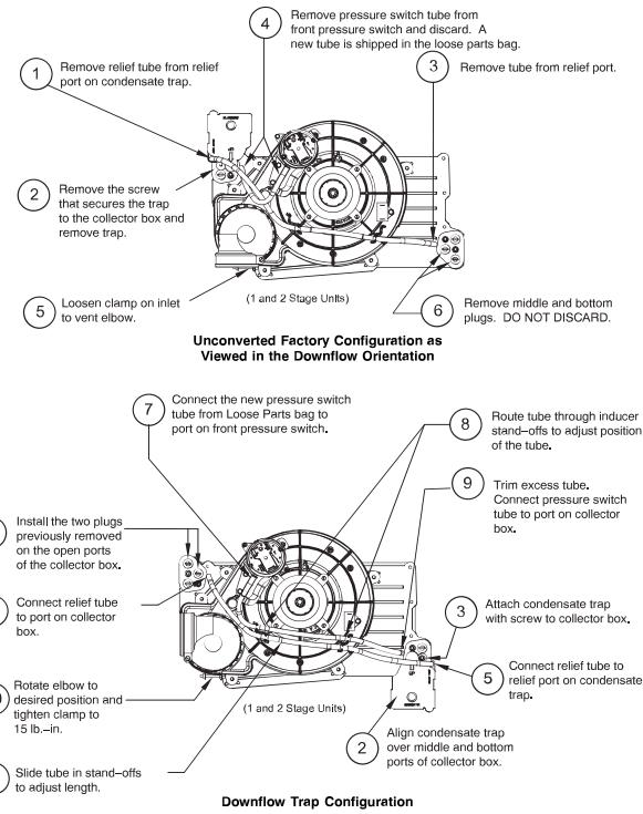
**Fig. 9 – Downflow Trap Configuration**
