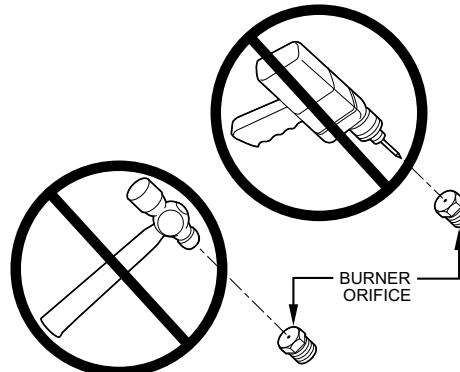
**Fig. 62 – Orifice Hole**
