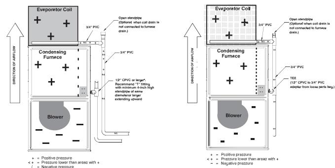
**Fig. 12 – Example of Field Drain Attachment**
