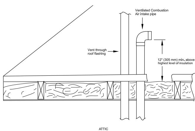
**Fig. 47 – Vent Terminations for Vented Combustion Air**
