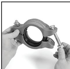
Disassemble coupling by loosening the nut on the coupling bolt only. Loosen nut to end of the bolt and swing out of slotted hole. Remove the gasket.
