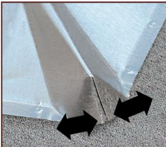
If pitch adjustment is needed, push the flange hips in to increase pitch, pull the flange hips out to decrease the pitch.
