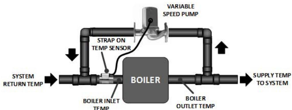
A strap on temperature sensor measures boiler inlet temperatures. This temperature signal is sent to a variable speed pump that will ensure boiler inlet temperatures are always greater than the factory by-pass kit set point of 120°F.
