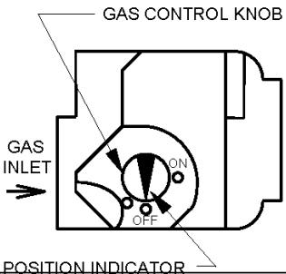
7. Rotate gas control knob clockwise
