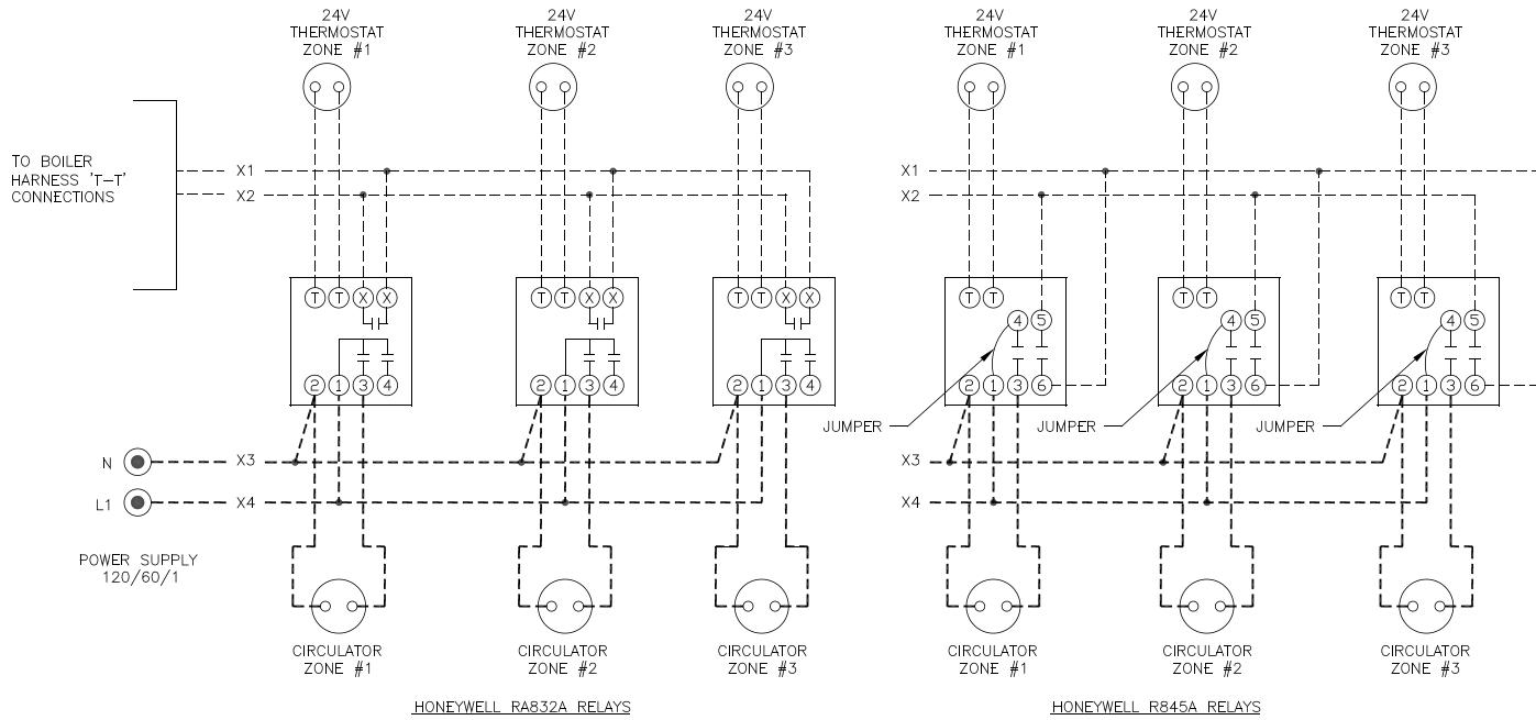
Figure 9-4: Wiring Schematic, Zone Circulators
