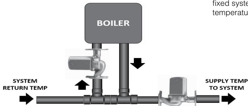
This is an improvement over simple by-pass piping to reduce condensation. Again this is a fixed system. It can not adapt to variations in temperature and flow.
