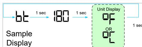
In order to view an instantaneous value, [i.e. instantaneous flame current.] User can press and hold either Up ↑ or Down ↓ key in operating mode
