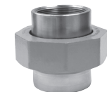
Fig. S1A High Speed Union 3,000 psi cwp – 4,500 psi test Size Range: 1" – 3"
