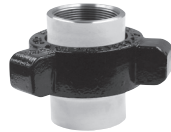
Fig. 100C Threaded Ends – Lug Union 1,000 psi cwp – 1,500 psi test Size: 2"
