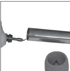
Clean any debris from inside of tube. Deburr or ream inside and outside of tube.
