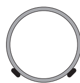
1c Two cables in 4 and 8 o'clock positions
