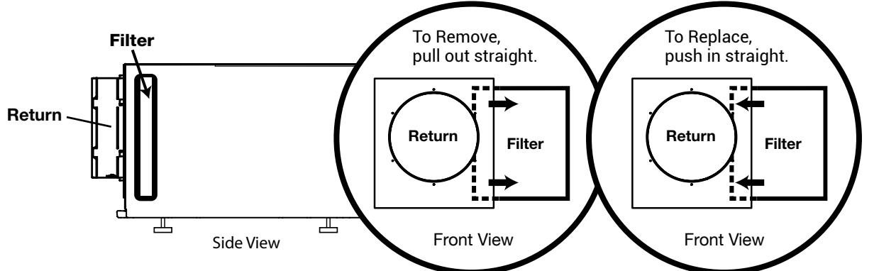
Step 3: Replace filter door ensuring the opening is fully covered.
