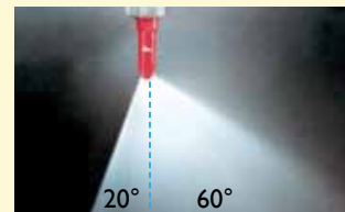
Band spraying in orchards/vineyards
