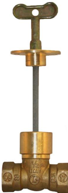
The C-67 AGA Gas Valve is for use on any gas fireplace or appliance. Using the included operating rod, the installer can install the valve from 1" to 14" depth, allowing it to be installed "below-the-joist," eliminating fittings and installation time. The C-67 Gas Valve is also used as a shutoff for any gas burning appliance.
