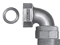
Quarter bend coupling Female Mueller Coupling thread x PJ for CTS O.D.* tubing
