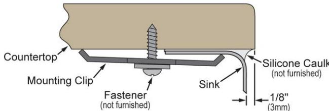
Designed to affix to the underside of any solid surface countertop.
