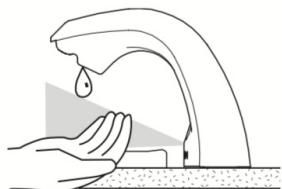
As the user's hands enter the beam's effective range, the beam is reflected back into the sensor receiver and activates the solenoid valve allowing a single soap application to flow from the spout.
