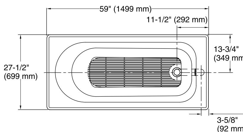
No change in measurement if connected with drain illustrated. (K-7161-AF)
