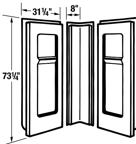
**General:** Furnish and install as shown on plans, 38" neo-angle shower, DURAWALL® Shower Walls Model 738C, as manufactured by E.L. Mustee & Sons, Inc. Shall be 3-piece, molded fiberglass wall with minimum thickness of 125 mils and mounts direct-to-studwalls. Includes center panel with molded-in shelves and two side panels with molded-in shelf. Self aligning panels use a tongue-and-groove connection. Shall meet ANSI Z 124-2011.2. Color: White.
