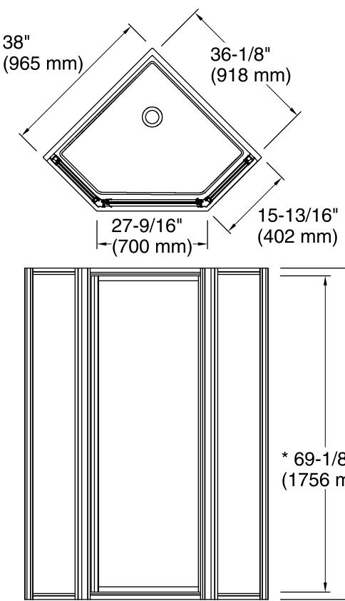
**Note:** Dimensions are taken on centerline of curb/threshold at the rough opening.
