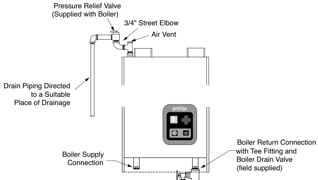
**Fig. 5A: Pressure Relief Valve and Boiler Drain Valve Installation (Models PT 175-399)**
