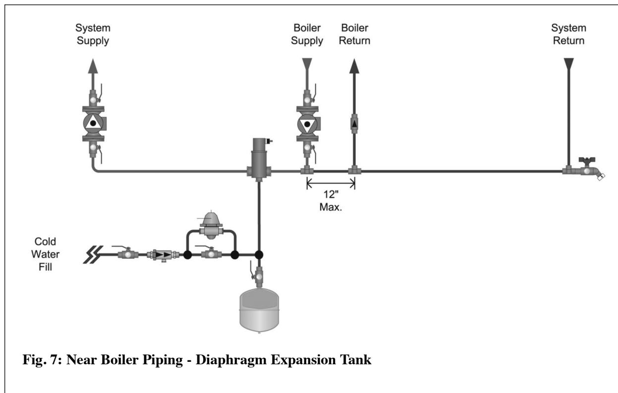
**Fig. 7: Near Boiler Piping - Diaphragm Expansion Tank**
