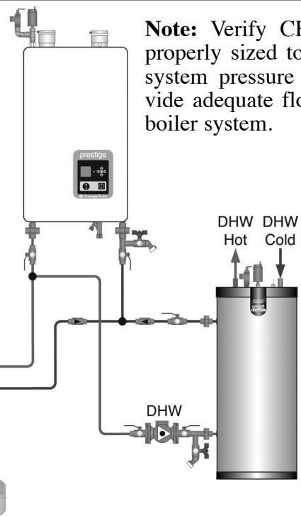
**Note:** Verify CH circulator is properly sized to overcome the system pressure drop and provide adequate flow through the boiler system.
