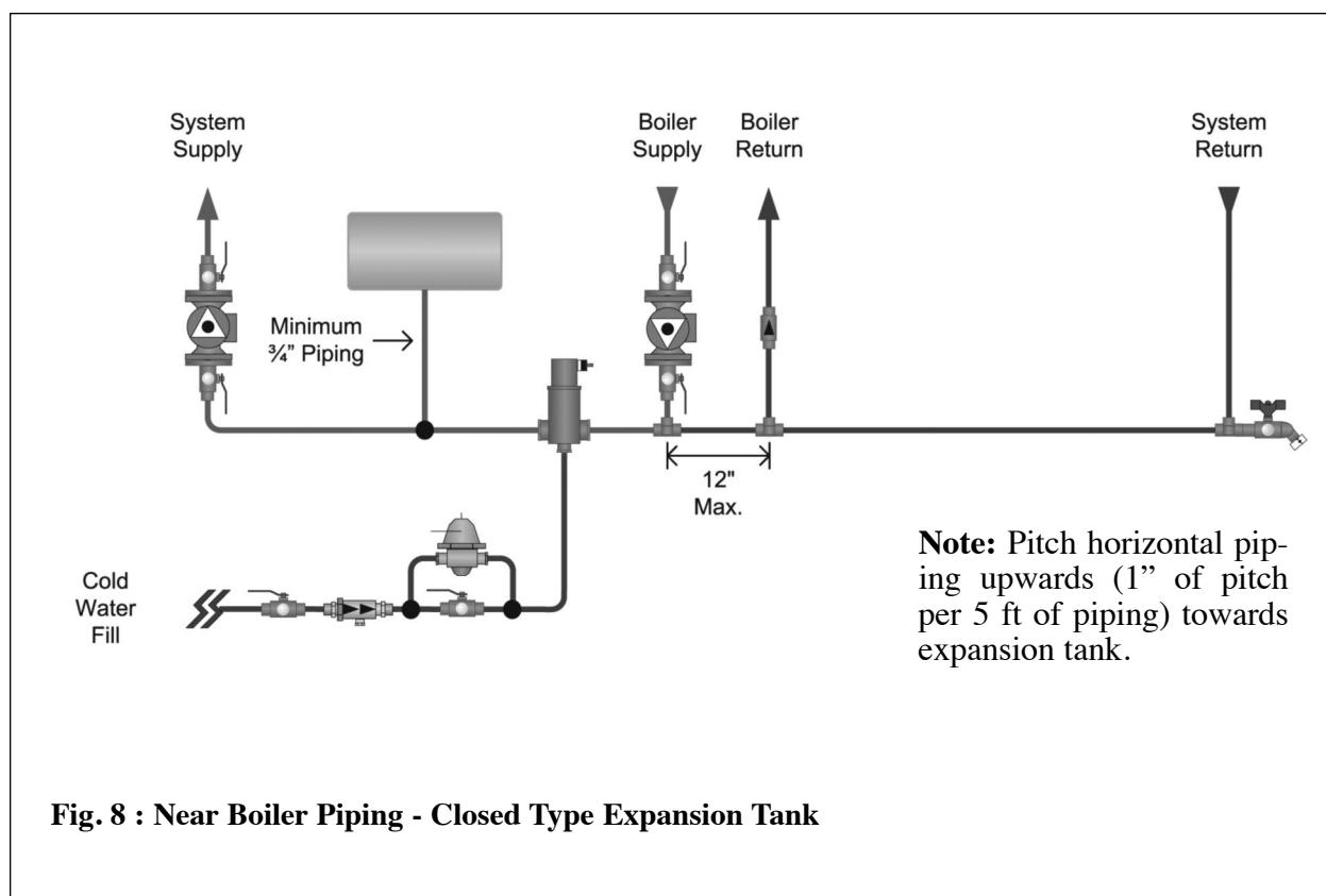
**Fig. 8 : Near Boiler Piping - Closed Type Expansion Tank**
