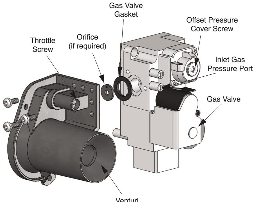
**Fig. 16: Gas Valve / Venturi Assembly - PRESTIGE Solo 60/175/250**
