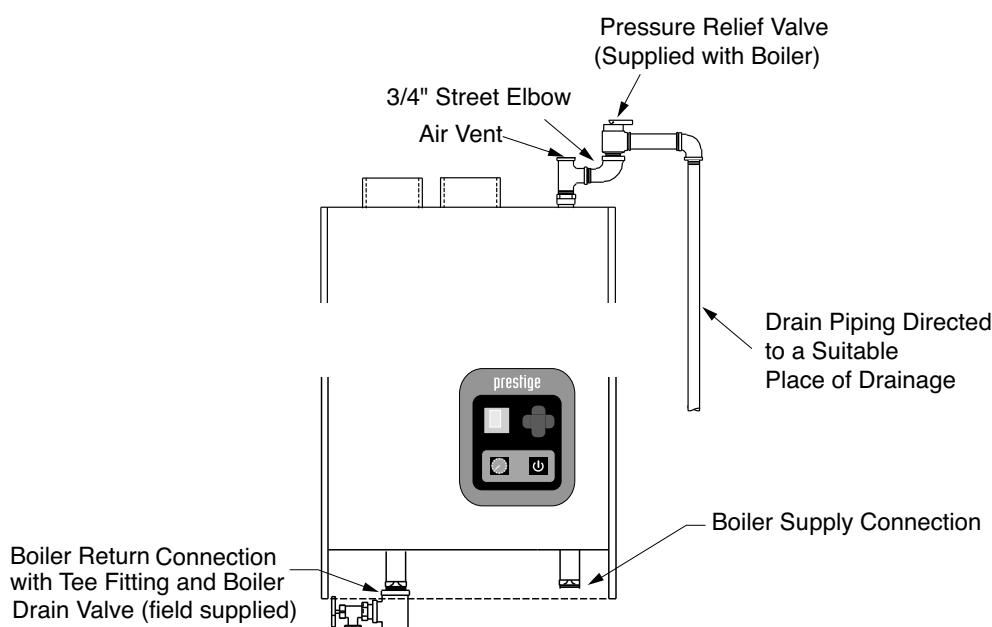
**Fig. 5B: Pressure Relief Valve and Boiler Drain Valve Installation (Model PT 60)**
